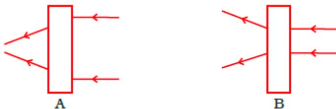
The given figures show the path of light through lenses of two different types, represented by rectangular boxes A and B. What is the nature of lenses A and B?
